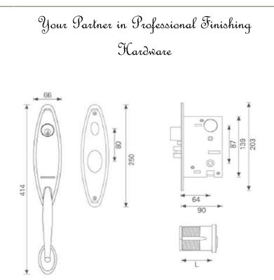
COMPLETE WITH: 64 OR 70MM BACKSET, U.S. MORTISE LOCK CASE GRAB HANDLE SET IN EXTIRIOR MORTISE THREADED CYLINDER SCREW PACK & DECORATED COVER PLATE LEVER OR KNOB, 8X8MM SPLIT TYPE SPINDLE KNOB WITH 4MM SPINDLE
