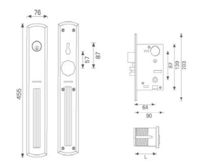
COMPLETE WITH: 64 OR 70MM BACKSET, U.S. MORTISE LOCK CASE GRAB HANDLE SET IN EXTIRIOR MORTISE THREADED CYLINDER SCREW PACK & DECORATED COVER PLATE LEVER OR KNOB, 8X8MM SPLIT TYPE SPINDLE KNOB WITH 4MM SPINDLE
