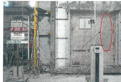
Photo 5: The unexposed face of the specimen after a heating period of 120 minutes.
