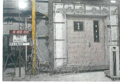
Photo 1: The unexposed face of the specimen before the test.
