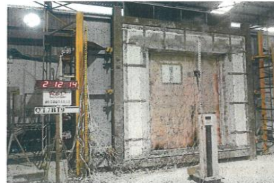
Photo 6: The unexposed face of the specimen after the test.
