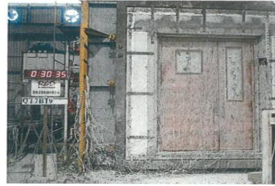
Photo 2: The unexposed face of the specimen after a heating period of 30 minutes.
